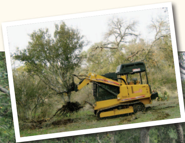
The skid steer with the grappling attachment plucks persimmon out of the ground.
